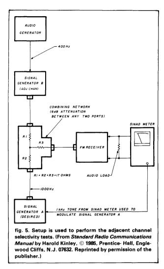
jacent channel and measures the result. This is the test we selected and performed to determine selectivity.
